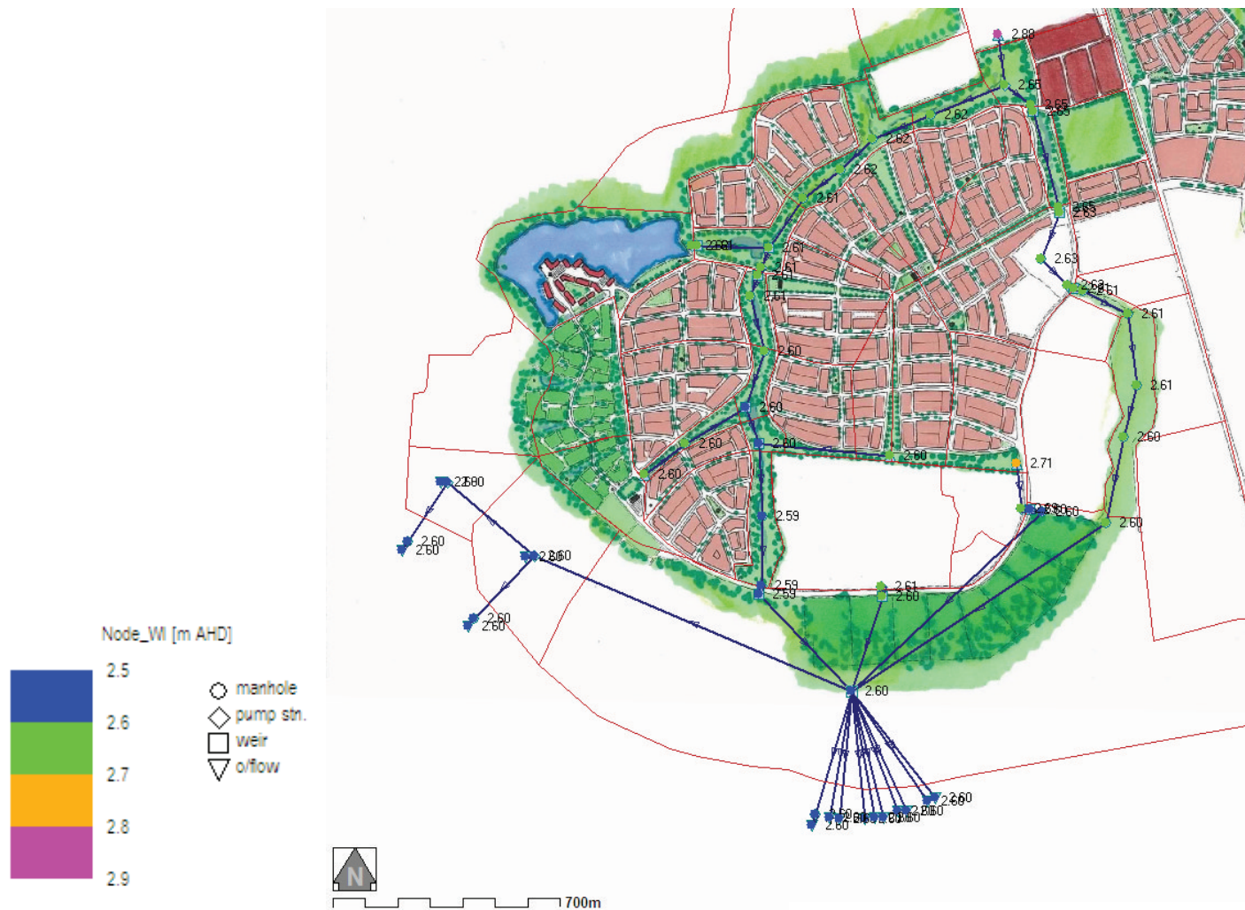
Figure 18. Peak Water Levels, Scenario 2 Increase in Rainfall 10% Increase in Tailwater 0.91 m
