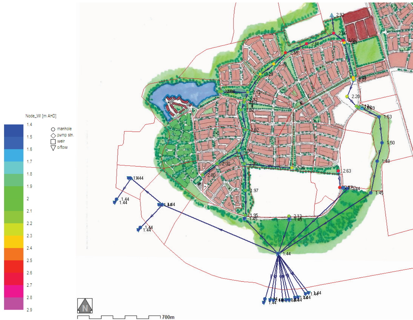
Figure 5. Peak Water Levels Scenario 1 Increase in Tailwater 0.18 m
