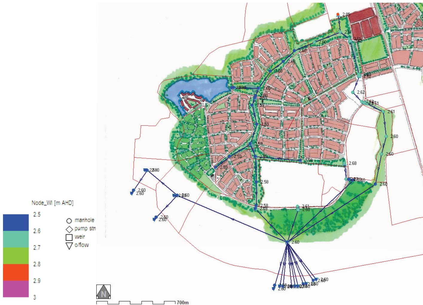
Figure 17. Peak Water Levels, Scenario 2 Increase in Tailwater 0.91 m
