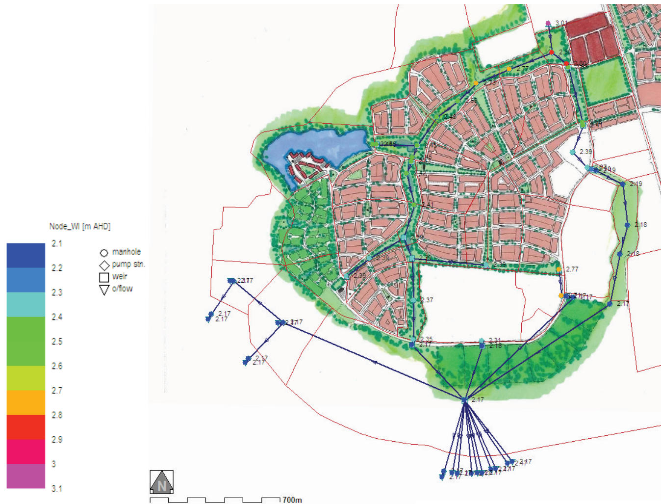
Figure 11. Peak Water Levels, Scenario 1 Increase in Rainfall 30% Increase in Tailwater 0.91 m
