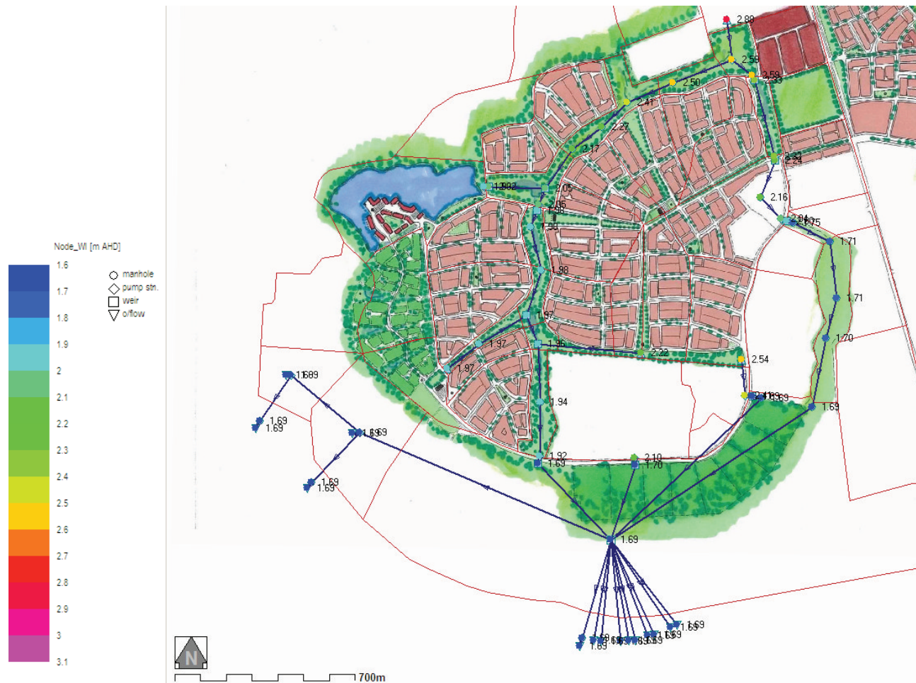
Figure 12. Peak Water Levels, Scenario 2 Increase in Rainfall Hydrograph 10%
