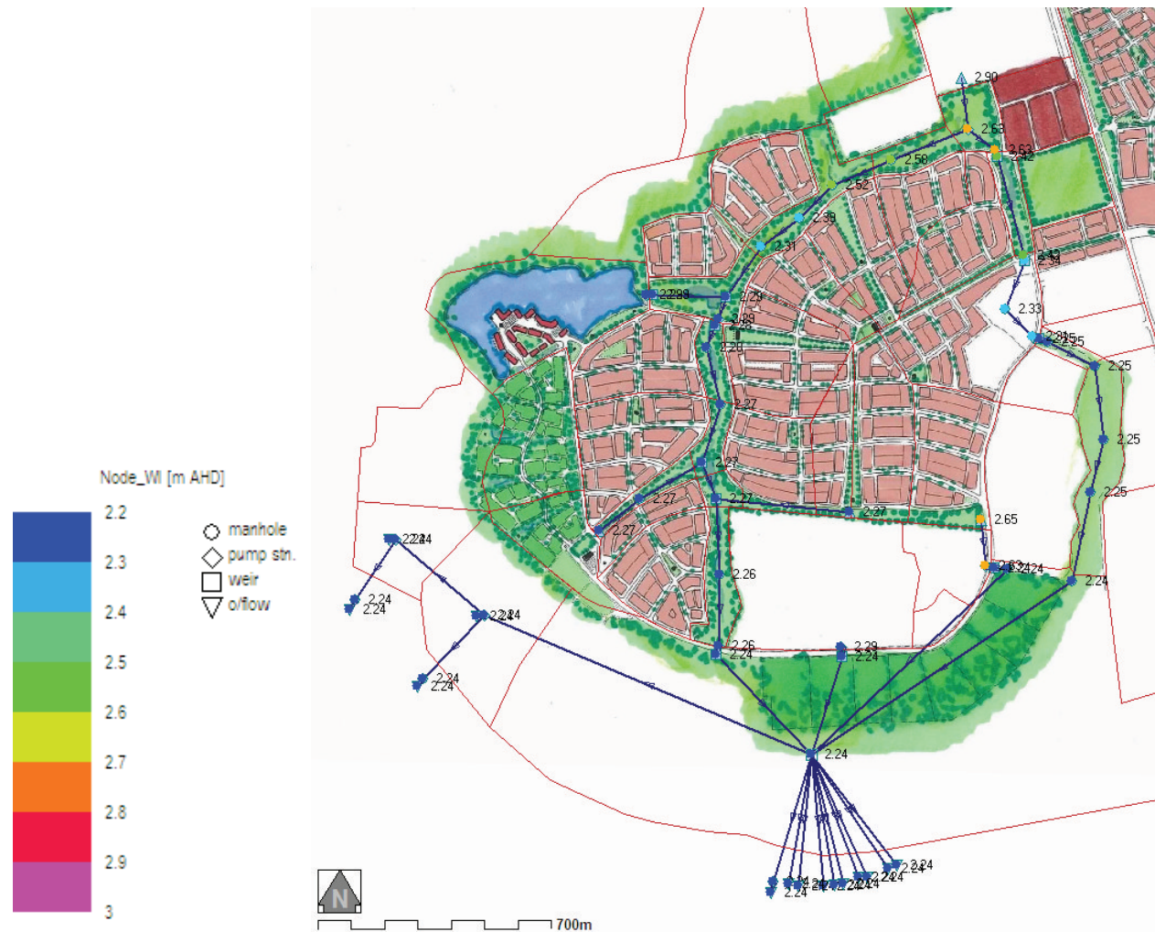
Figure 19. Peak Water Levels, Scenario 2 Increase in Rainfall 20% Increase in Tailwater 0.55 m
