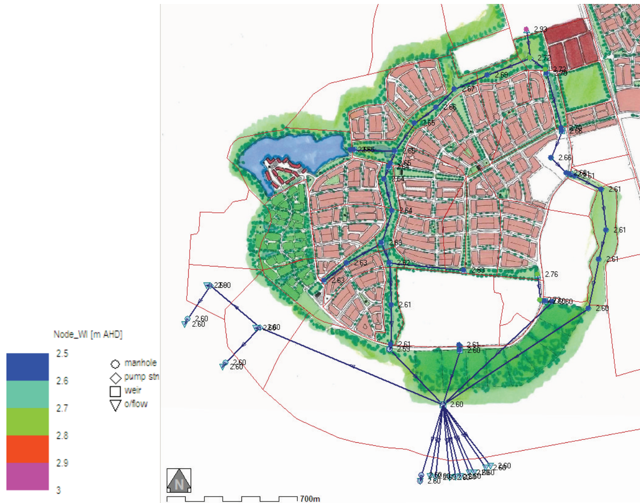
Figure 21. Peak Water Levels, Scenario 2 Increase in Rainfall 30% Increase in Tailwater 0.91 m
