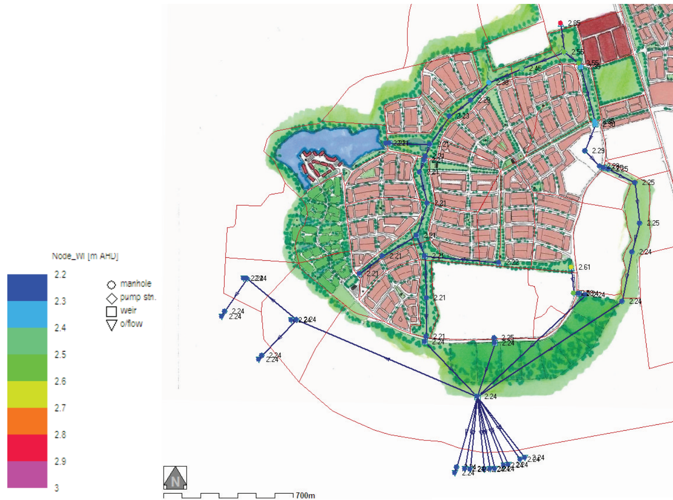
Figure 16. Peak Water Levels, Scenario 2 Increase in Tailwater 0.55 m
