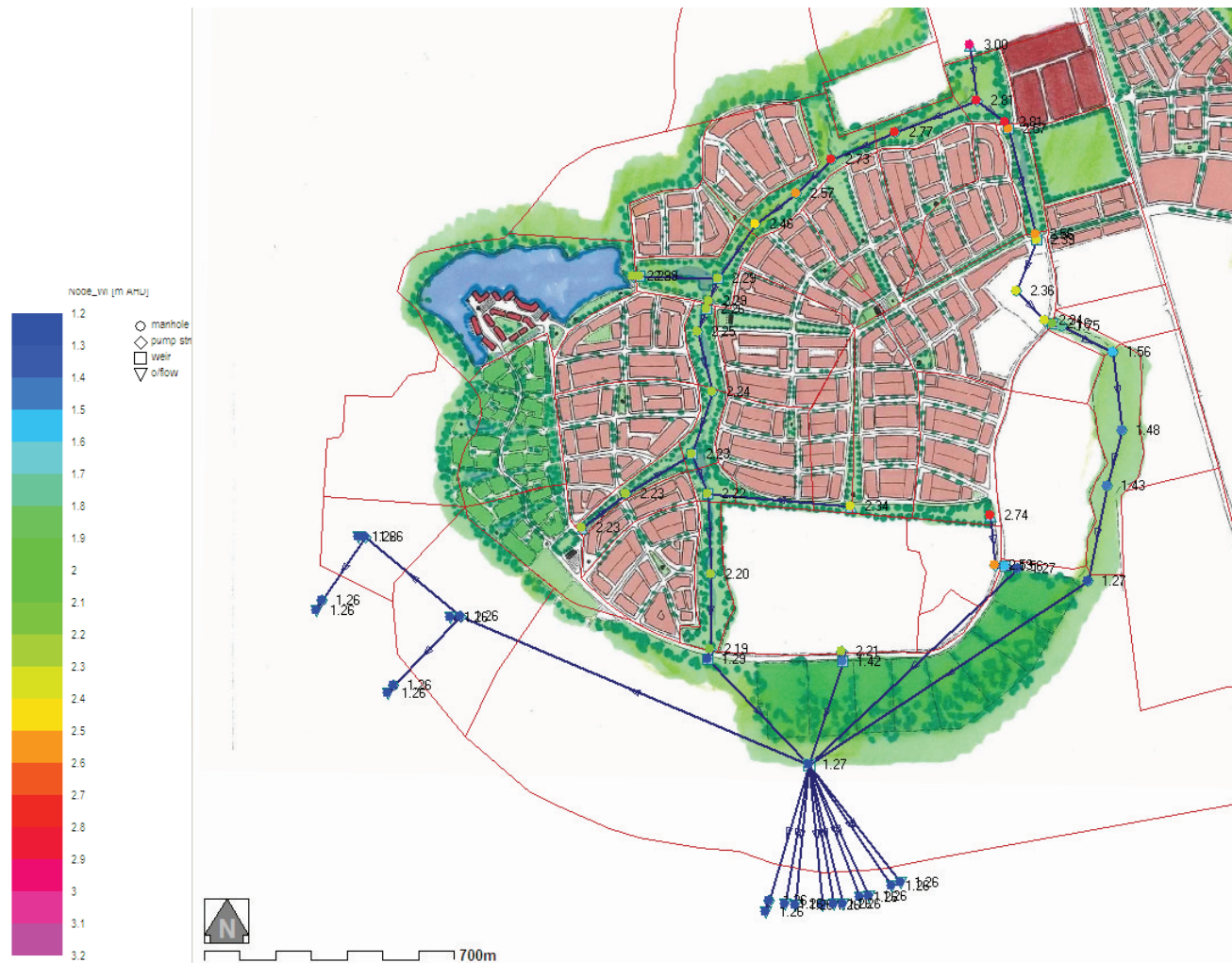
Figure 4. Peak Water Levels, Scenario 1 Increase in Rainfall Hydrograph 30%
