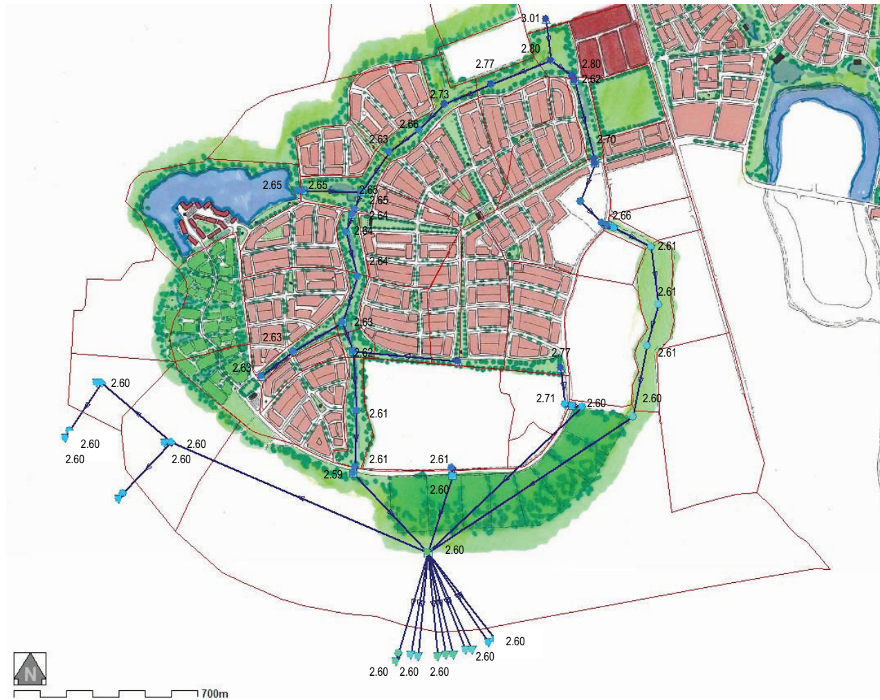
Figure 23. Maximum Peak Water Levels, Combination of Scenarios 1 and 2 Increase in Rainfall 30% and Increase in Tailwater 0.91 m
